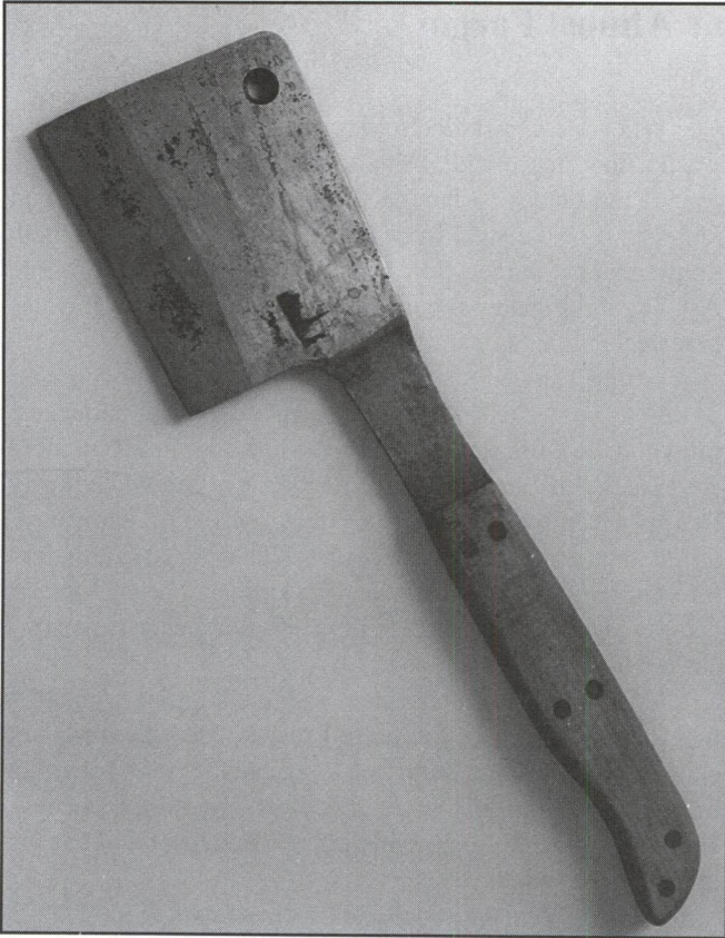
This old Berry hatchet sports steel from a road grader. Though the author says its edge geometry is not as good as other Berry pieces, it still does the job.
