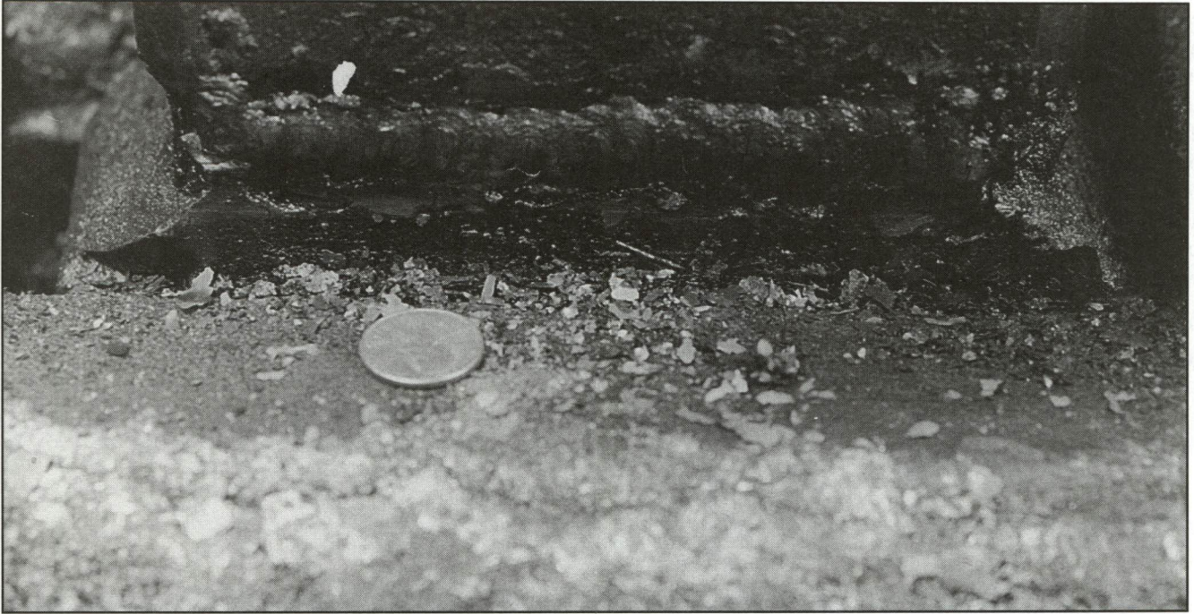
The fine flakes indicate the steel was forged at a lower temperature more conducive to a high-performance blade.
