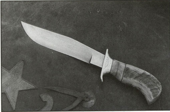
The author forged his Iron Mistress from 52100 steel. The guard is brass, the handle is sheep horn.
