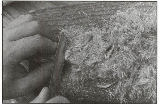
The bronzed blade slightly outcuts the unbronzed blades in the author's cutting.
