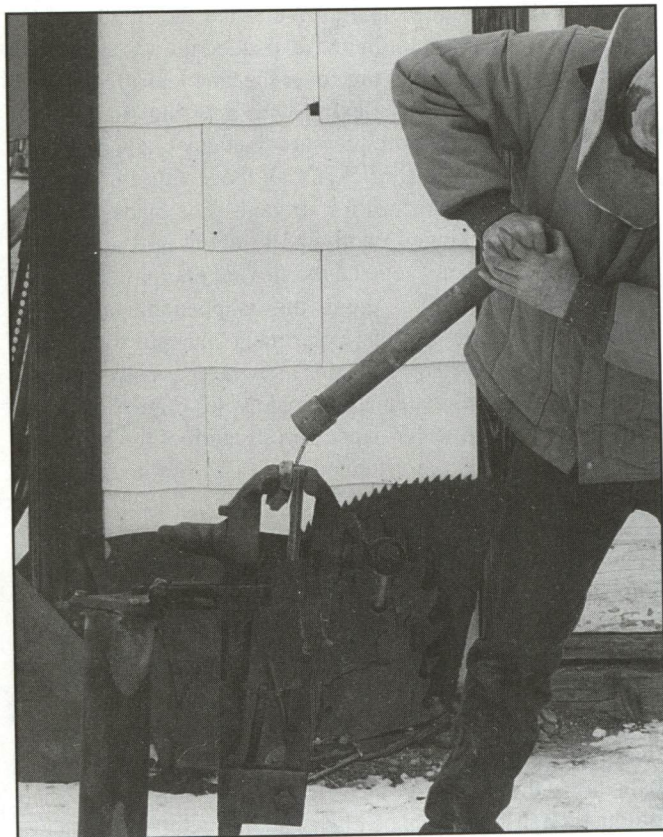
The frozen blade was strong and flexed to 90° without cracking.
