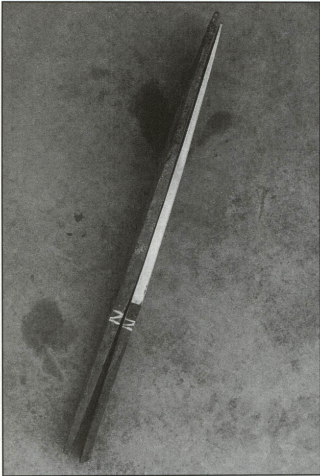
An overhead view of the two blades. Note how much thicker the unground forged blade is.
