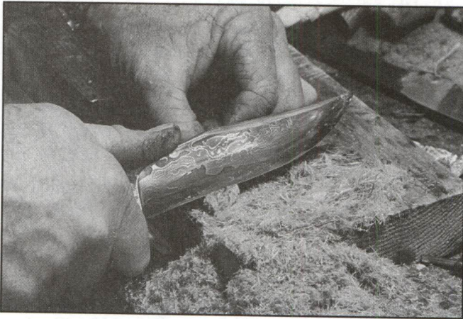
The author said the freeze-quenched blade cut better than any Damascus blade he's ever tested.
